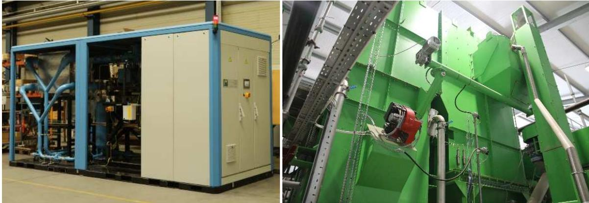
Left: ORC UHT 111/90kWe – Right: fluidized bed biomass boiler
