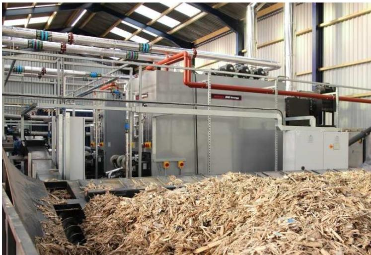
Richard Threlfel, owner of Crossfields Farm and co-owner of the project says: "Unlike it may be expected, the use of the low temperature isn't a real disadvantage for the drying process. The right air flow which blows the warm air through the 4ft packed woodchips is also important. The drying result is better than for many high temperature driers. Even wood shavings can easily be dried in this installation. The current set-up gives the best fit between power production and drying requirements."
